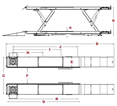
Note: An air supply (minimum: 30 psi / 3 CFM) is required for the safety-lock mechanisms to disengage. It is solely the responsibility of the end-user to provide, install and maintain the air supply.
